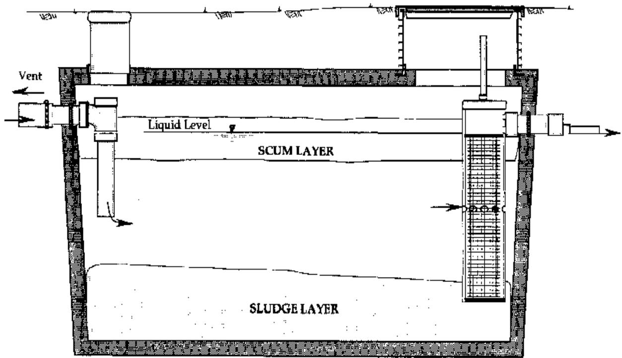
Figure 2 - Typical Septic Tank with Effluent Filter
